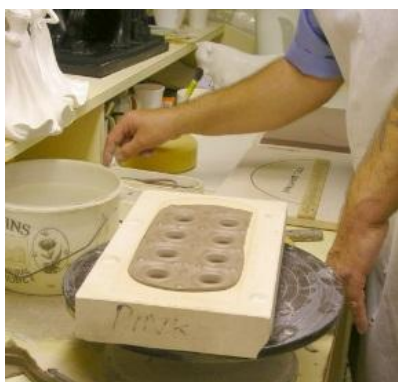
time for the thimbles to be unmoulded
