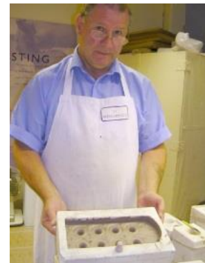
raw clay thimbles in their picture mould with a pink thimble to show the colour they will become
