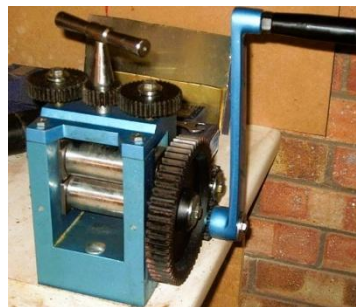
stamp mill used for making silver sheets thin enough for creating RN thimbles
