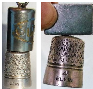
examples of different Elfin thimbles attracting a magnet, showing their "with steel reinforced ends"
