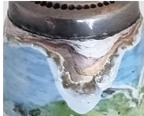
enamelling damage on a sterling silver thimble
