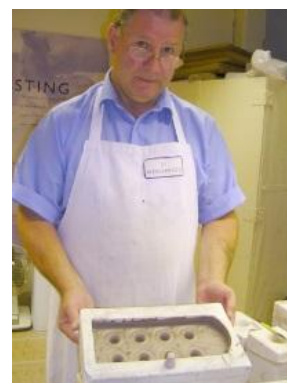
raw clay thimbles in their picture mould with a pink thimble to show the colour they will become
