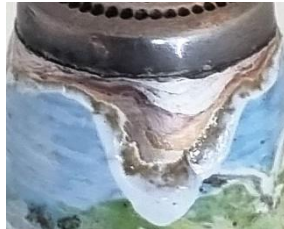
enamelling damage on a sterling silver thimble
